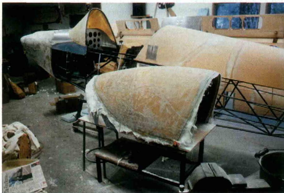
The compound curves of the custom Beryl canopy proved tricky for this scratch builder, but a cleverly-designed centerline canopy top solved the problem and provides some solar protection on sunny flights.
