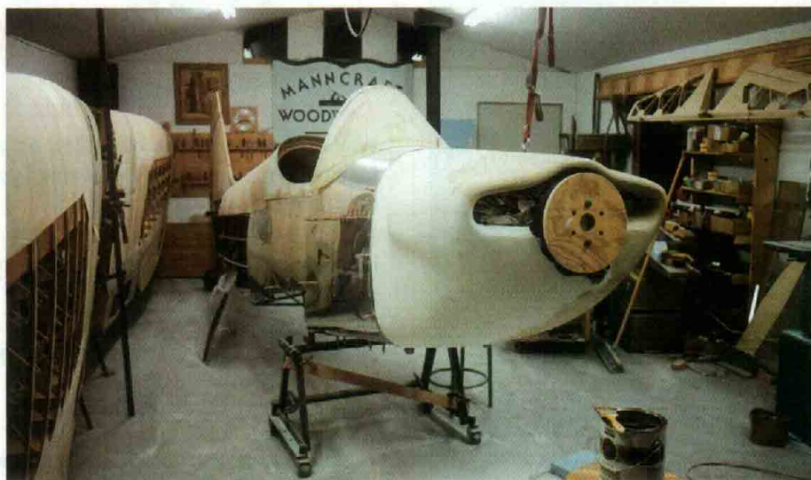
The variety of materials used in the construction of the Beryl was part of the challenge. Steel tube, wood, aluminum, and fiberglass all contribute to the aircraft's structure.
