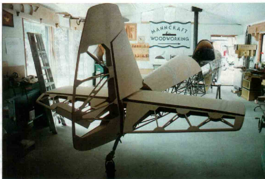
The variety of materials used in the construction of the Beryl was part of the challenge. Steel tube, wood, aluminum, and fiberglass all contribute to the aircraft's structure.
