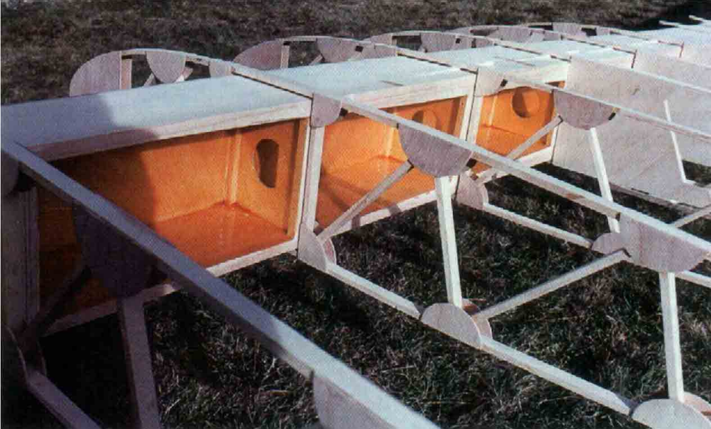
Since T-88 epoxy worked so well on the author's previous project—an Emeraude—he used it as the adhesive of choice on the Beryl's wood wings.
